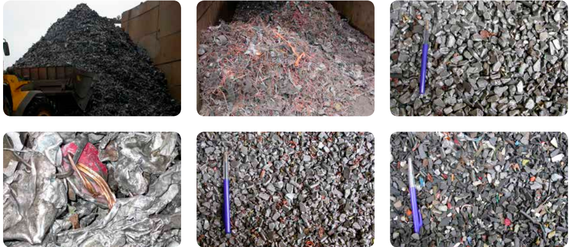
Figure 29: Impure quality recyclates created during physical separation of shredded cars (Reuter et al., 2005).
