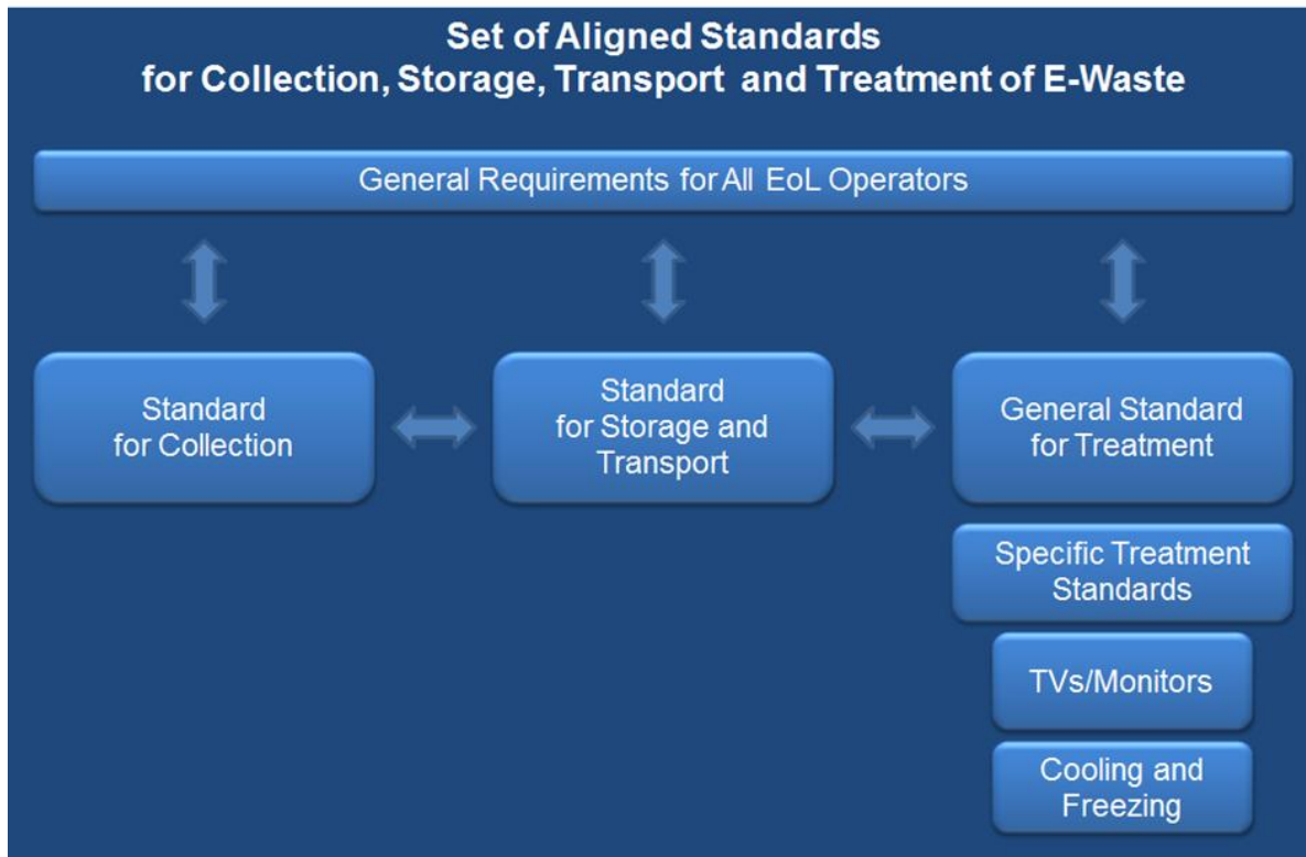
Figure 1: Example architecture of EoL standards covering the entire EoL chain of EEE
