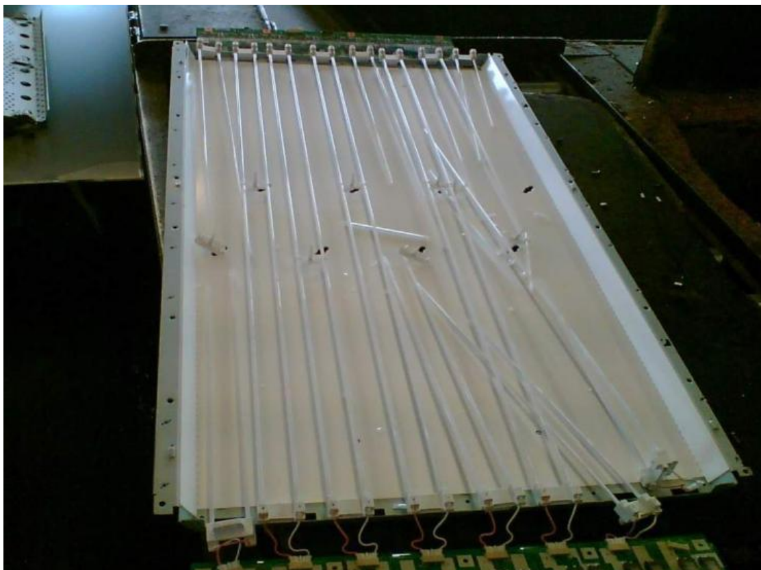
Figure 19: Rear part of a flat panel display with broken backlights 32
